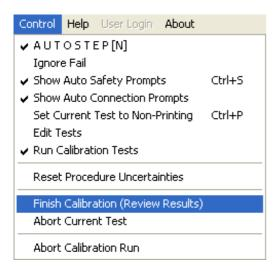
STEP 12 When the last test is reached, the test Review Screen is displayed - Click Next >> (if a message stating some tests are not completed appears, simply click YES to proceed)
