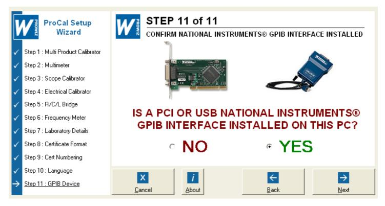
Step 11 - Set ProCal GPIB support for National Instruments Internal (PC Card) and External (USB) devices.
