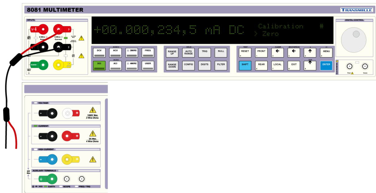
Figure 5 – DC Current Zero Connection
