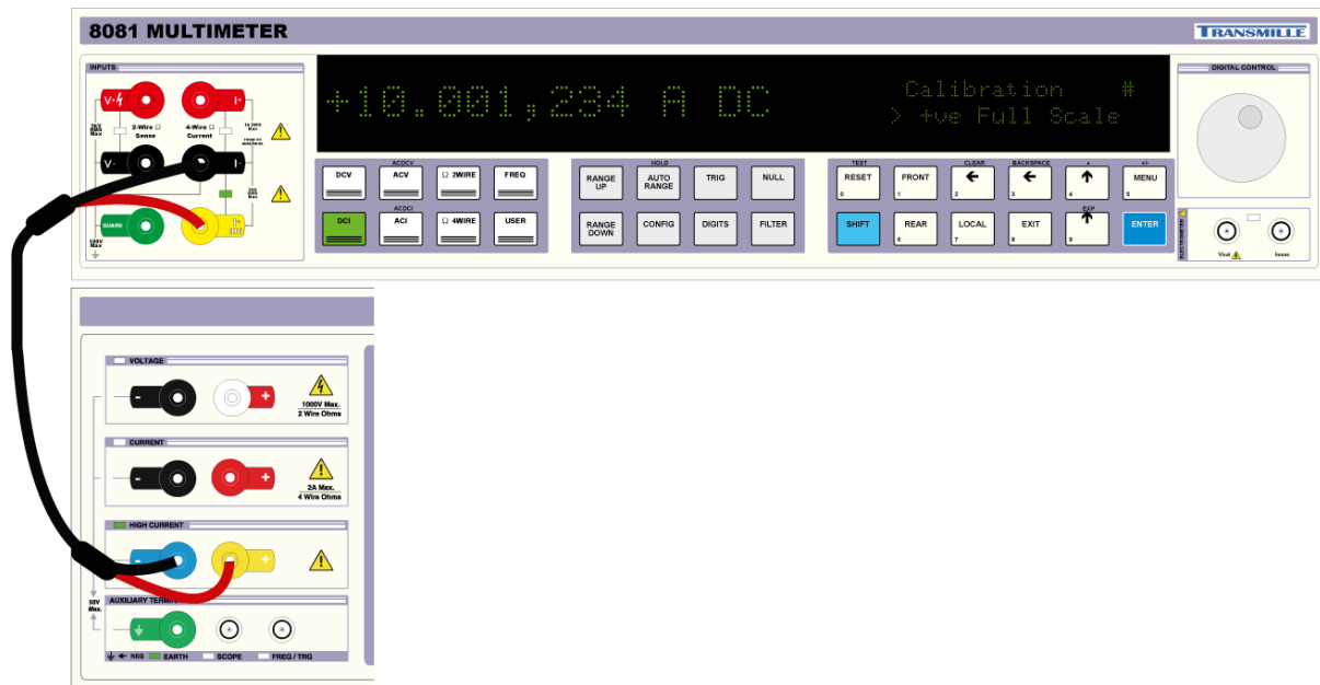
Figure 6 – DC Current Connection (up to 1A)
