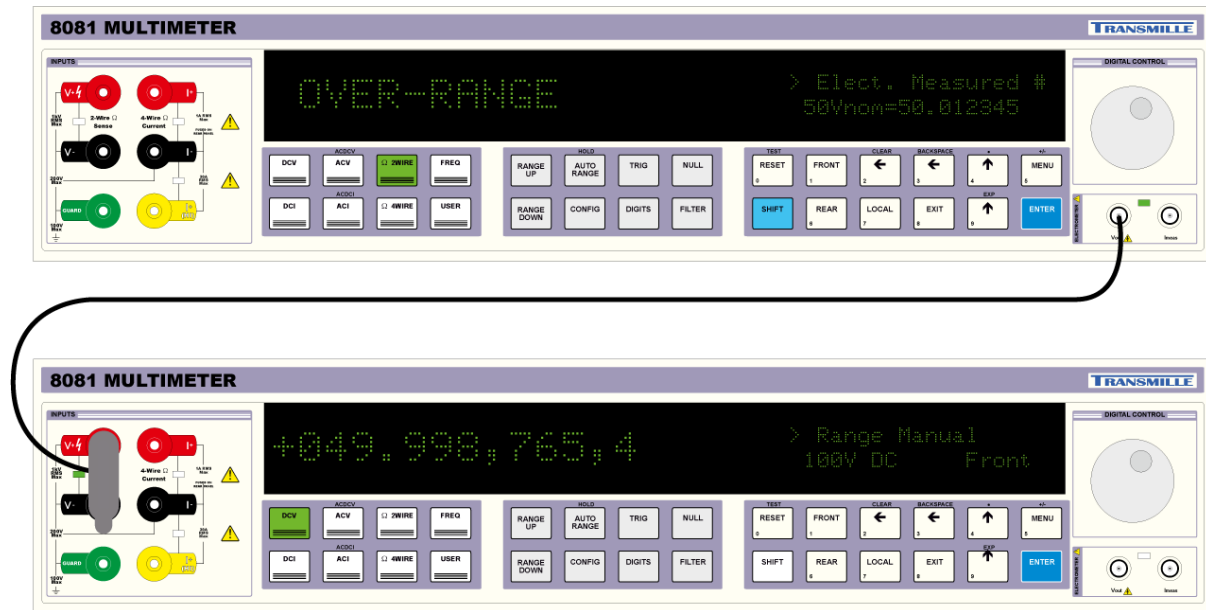
Figure 18 – Connection for Electrometer Voltage Output measurement
