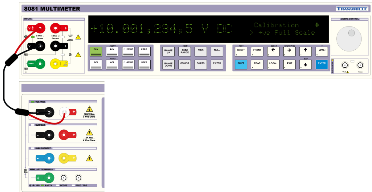
Figure 3 – DC Voltage Connection using Calibrator
