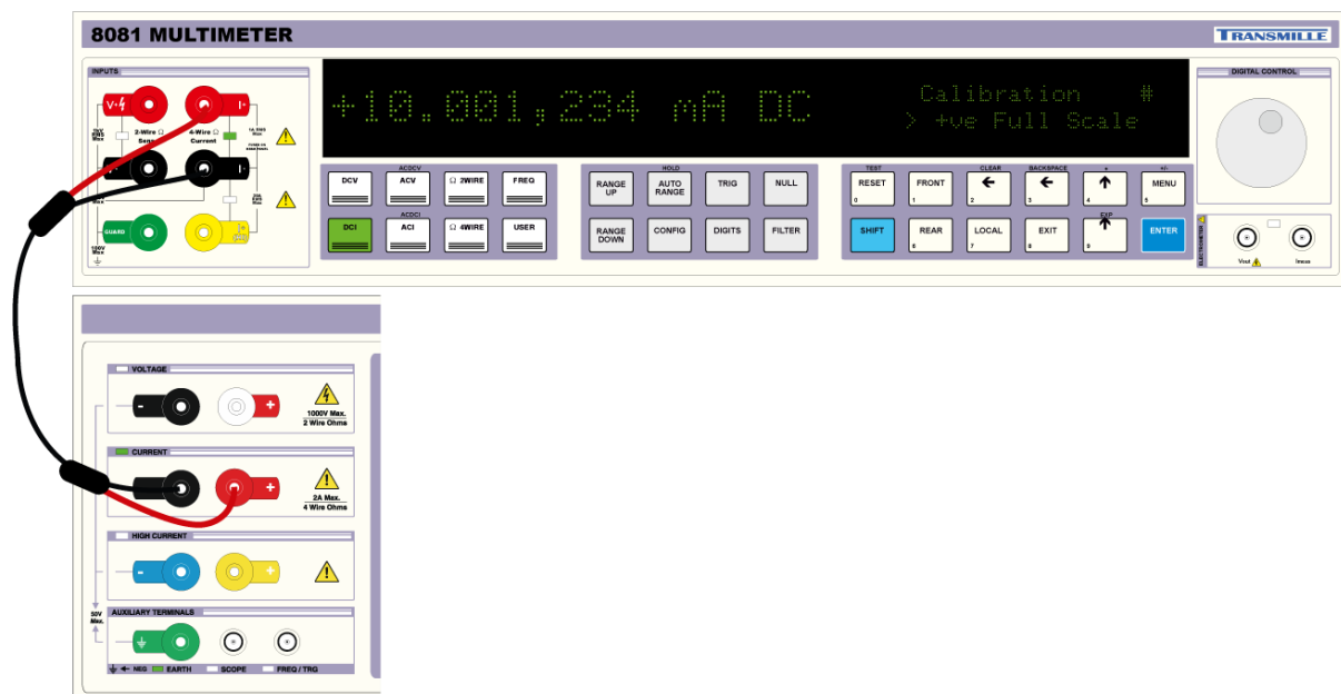
Figure 7 – DC Current Connection (from 1A to 30A)
